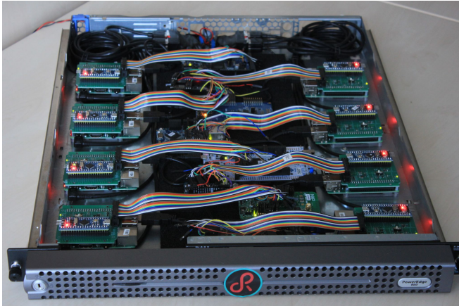
Figure 4: One rack of the RIOT HiL testbed used for our benchmarks.
